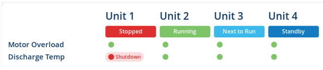
Figure A.3.7.4 Unit Shutdown
