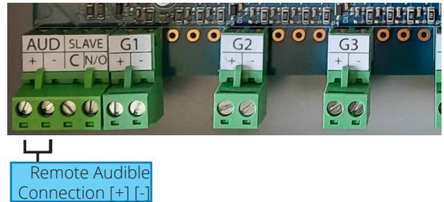
2.2.7 Alarm output fault relay connection (see figure 17)
