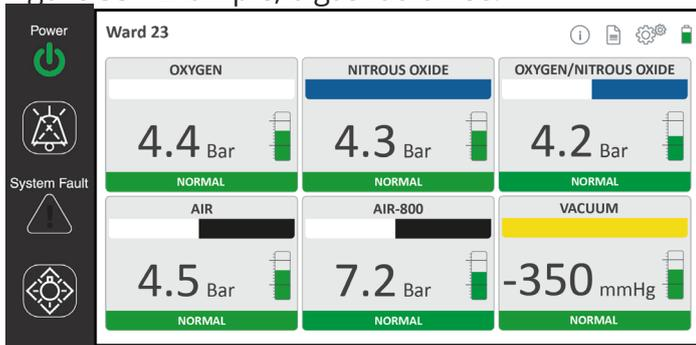
Press the TEST switch and check all gas service indicator bars flash at the same rate, the audible warning sounds and the system fault LED flashes.
