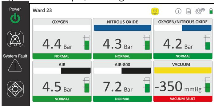
4.6.3 Pressure Sensor. Vacuum fault reset.
