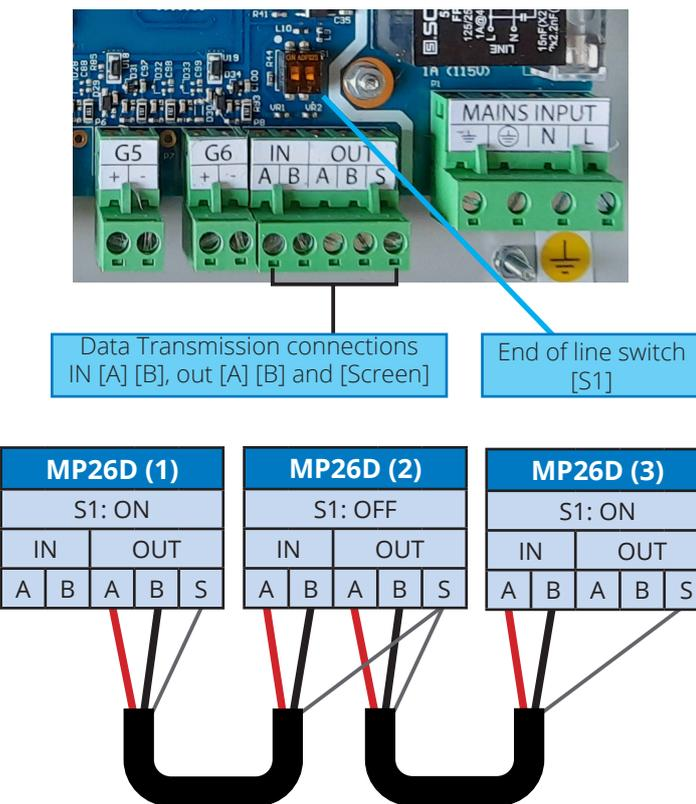
Note - "S" terminal is for connecting the screen cable.
