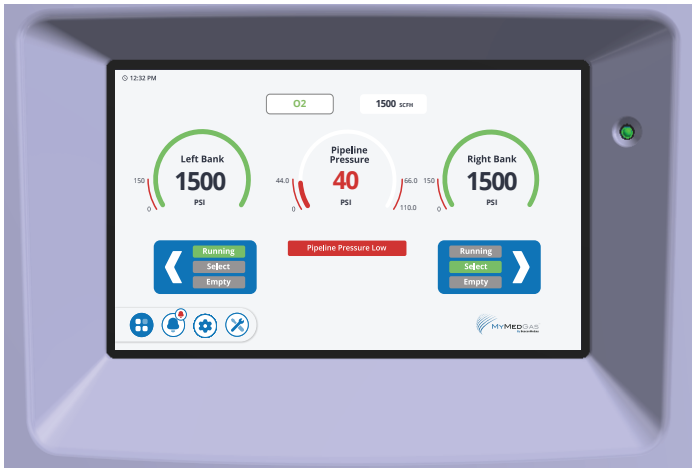
Figure 23 - Low Line Pressure Fault.
