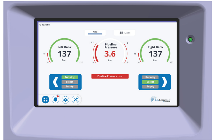
Figure 24 - Low Line Pressure Fault.
