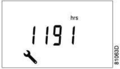
Example of running hours on display since last service.
