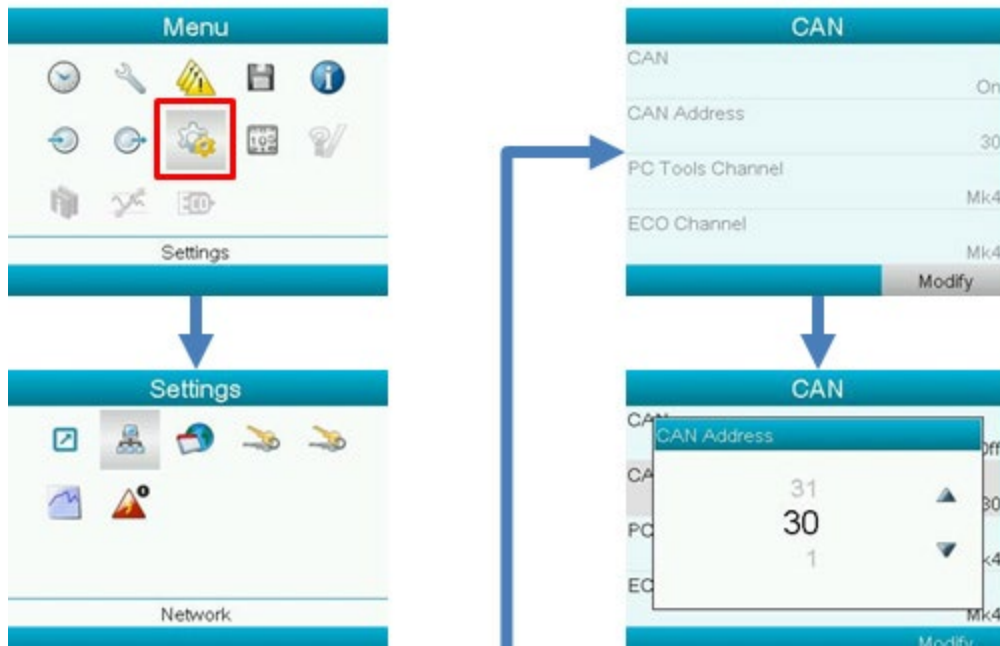
Figure 8-17; Central controller – CAN settings
