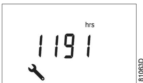
Figure 8-7; Example of running hours on display since last service
