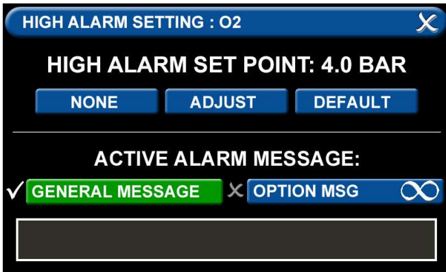
Figure 96: High Alarm Settings Tab
