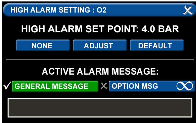
Figure 42: High Alarm Settings Tab
