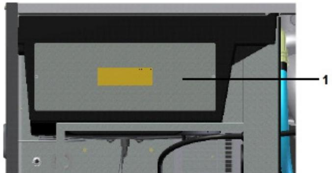
Remove dirt from the coolers with a fibre brush. Brush in the direction of the cooling fins.
