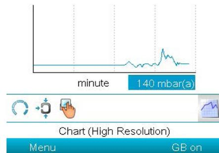
When Chart (High Resolution) is selected, the chart shows the variation of the selected input (in this case the pressure) per minute. Also the instantaneous value is displayed. The screen shows the last 4 minutes.
