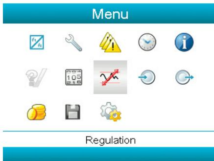
Using the scroll keys, move the cursor to the Event History icon (see above, section Menu icon). Press the enter key, the list of the last shut-down and emergency stop cases is shown.
