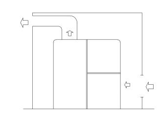
VENTILATION PROPOSAL: Standard Unit (See note 6) (Common ducting for multiple units is not allowed)
