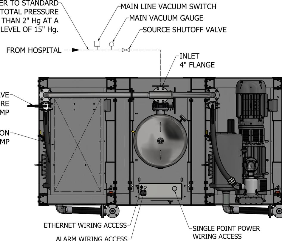
PIPE EXHAUST OUTSIDE, TURN DOWN AND SCREEN PER NFPA 99
