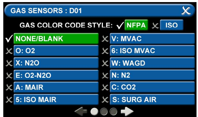
Figure 80: Gas Sensors Screen
