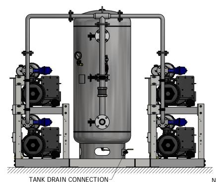
NO VIBRATION PADS-ARE NECESSARY AT THIS LOCATION
