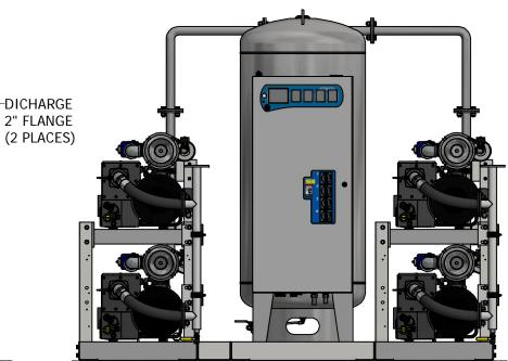
NO FOUNDATION OR INERTIA PAD IS REQUIRED (HOUSEKEEPING PAD IS OPTIONAL)
