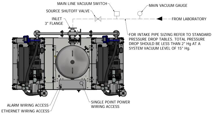
PIPE EXHAUST OUTSIDE, TURN DOWN AND SCREEN PER NFPA 99
