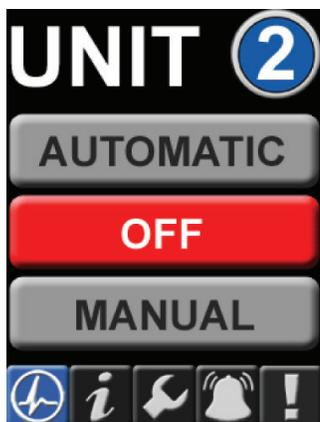
**Figure 3.3 Unit Screen - Off Position**
