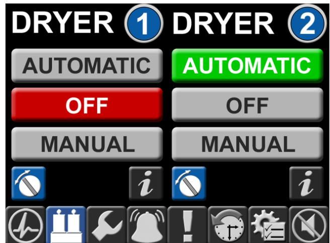
**Figure 3.7 Main Screen - Dryer Operation**
