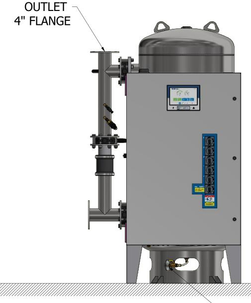
TANK DRAIN LOCATION CONTRACTOR SHALL PIPE TO FLOOR DRAIN
