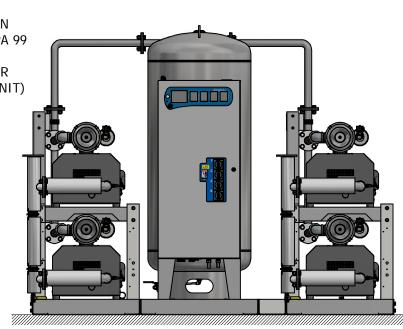
NO FOUNDATION OR INERTIA PAD IS REQUIRED (HOUSEKEEPING PAD IS OPTIONAL)
