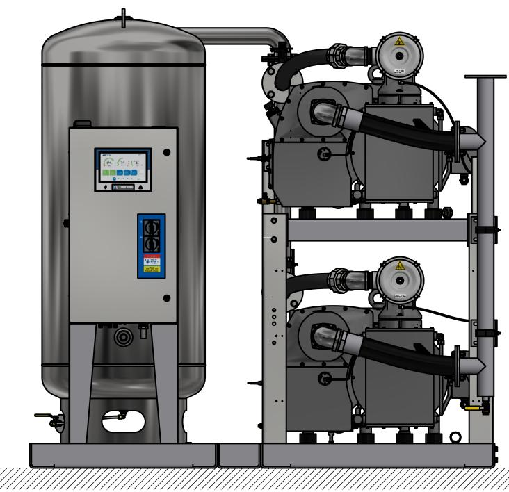
NO FOUNDATION OR INERTIA PAD IS REQUIRED (HOUSEKEEPING PAD IS OPTIONAL)
