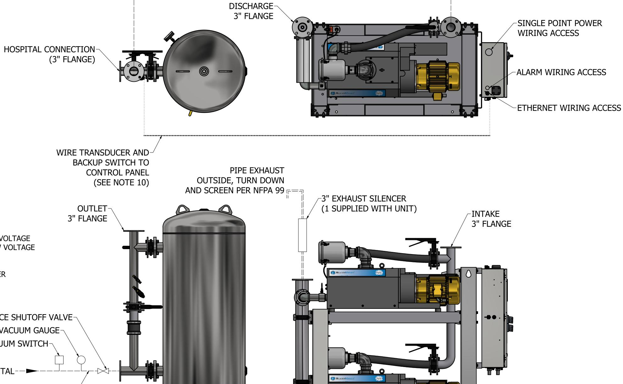
NO FOUNDATION OR INERTIA PAD IS REQUIRED (HOUSEKEEPING PAD IS OPTIONAL) DRIP LEG VALVE-
