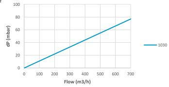
Note: 10" cartridge tested with air @ 20°C, 7 bar
