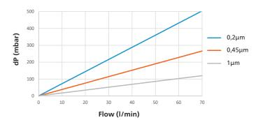
Note: 10" cartridge tested with water @20°C, 1,005 cP (typical flow rate)
