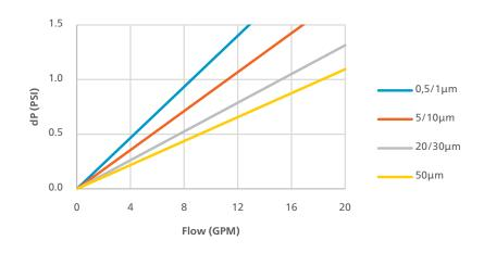
Note: 10" cartridge tested with water @ 68°F, 1.005 cP (typical flow rate)
