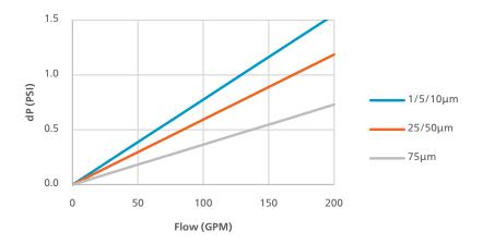
Note: 40" cartridge tested with water @ 68°F, 1.005 cP (typical flow rate)
