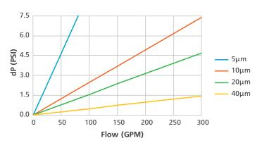
Note: 40" cartridge tested with water @68°F, 1.005 cP (typical flow rate)
