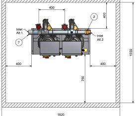
Recommended area around installation for operating and maintenance
