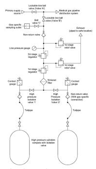
Note: ERM ECO based on a multistage pressure regulator, where 1st and 2d stage regulators combined into one unit.
