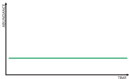
A normal baseline is flat, without peak and no drifts.
