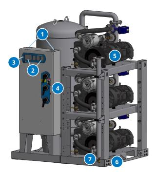
Single point vacuum inlet flange connection and receiver inlet positioned below receiver exit and piping to the pumps - extra protection against liquids/debris entering pumps.
