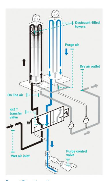
Dryer airflow schematic
