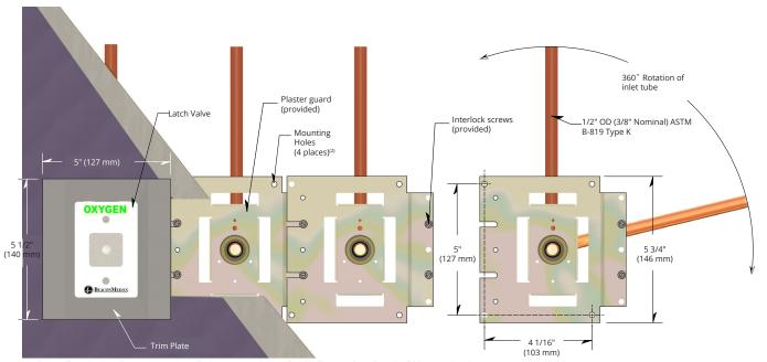
(1) When wallboard is less than 1/2" / 12.5 mm thick, as in consoles and headwalls, console outlets should be considered.
