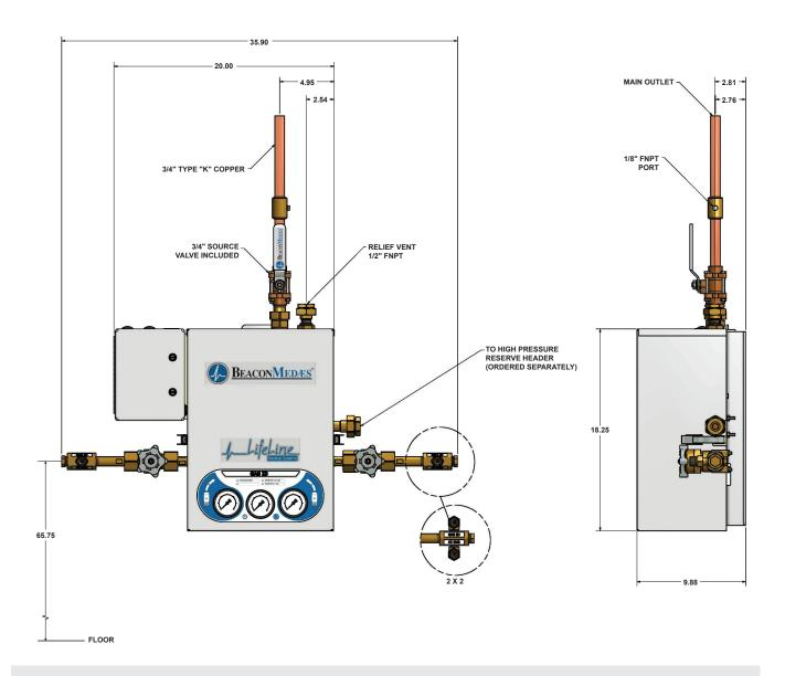
**Note:** The **Lifeline**® automatic changeover medical liquid manifold may be configured in 1 container (1 × 1) or 2 container (2 × 2)
