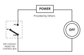
In this situation, both gas cylinder bank pressures are satisfactory (i.e. not empty). The dry contact inside the remote alarm box is in the Normally Closed position. The electrical circuit is open and the alarm device is NOT actuated.
