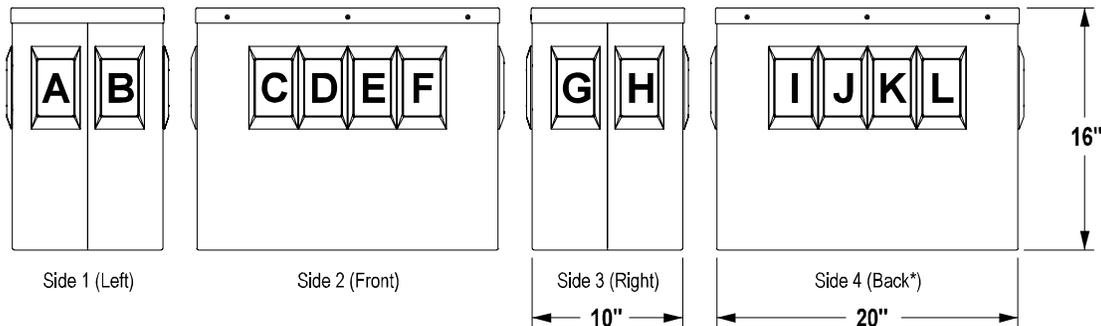
**\*NOTE: P/N 6-PED08-XX has a solid back panel. No future expansion in positions "I", "J", "K", or "L".**
