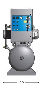
Notes: • Allow 36 inches in front of control panel for maintenance and ventilation, all other sides require 24 inches of clearance.
