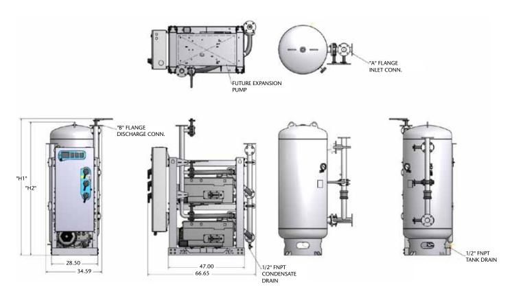
Notes: • Allow 36 inches in front of control panel for maintenance and ventilation, all other sides require 24 inches of clearance.
