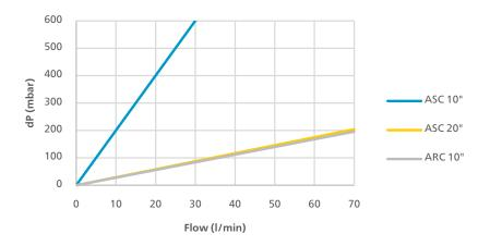
Note: 10" cartridge tested with water @ 20°C, 1.005 cP (typical flow rate)
